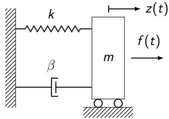
$f(t) = \text{input}$ ,  $z(t) = \text{output}$
