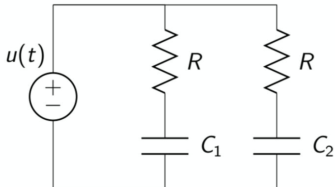
$$x_1(t) = v_{C_1}(t), \quad x_2(t) = v_{C_2}(t)$$
