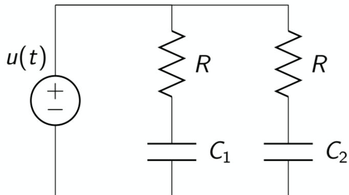
$$x_1(t) = v_{C_1}(t), \quad x_2(t) = v_{C_2}(t)$$
