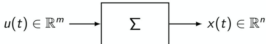
$$x^* = x(t) = \underbrace{e^{Ft} x_0}_{\text{ev. libera}} + \underbrace{\int_0^t e^{F(t-\tau)} Gu(\tau) d\tau}_{\text{ev. forzata}}$$
