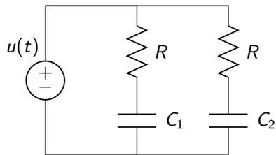
$$x_1(t) = v_{C_1}(t), \quad x_2(t) = v_{C_2}(t)$$
