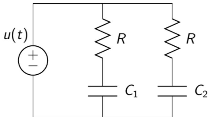
$$x_1(t) = v_{C_1}(t), \quad x_2(t) = v_{C_2}(t)$$
