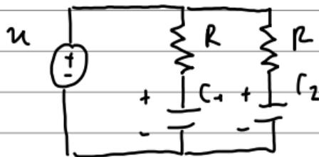
$$x_1 = v_{C_1} \quad x_2 = v_{C_2}$$
