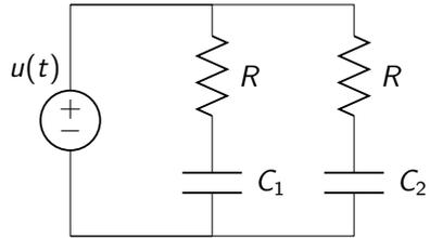
$$x_1(t) = v_{C_1}(t), \quad x_2(t) = v_{C_2}(t)$$
