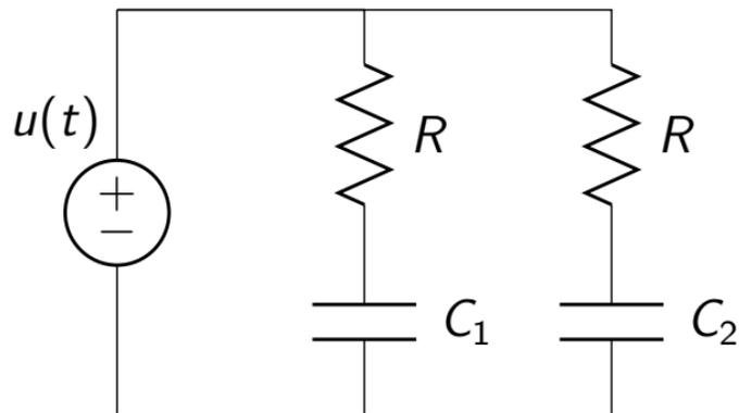
$$x_1(t) = v_{C_1}(t), \quad x_2(t) = v_{C_2}(t)$$
