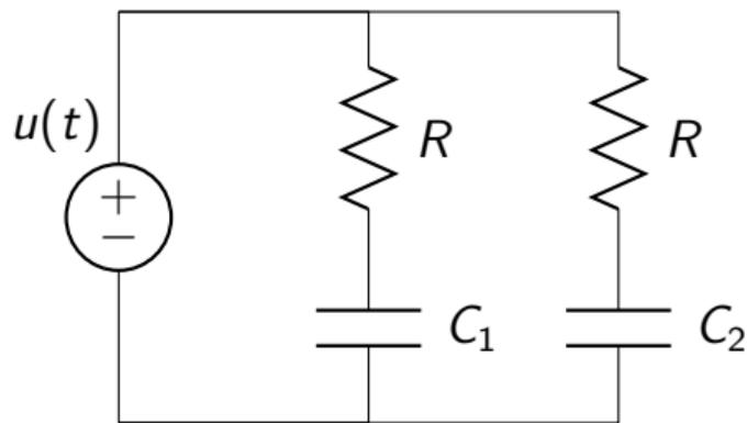
$$x_1(t) = v_{C_1}(t), \quad x_2(t) = v_{C_2}(t)$$
